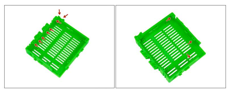
Slide **11x M3 square nuts** into the slots provided on the inside of the Duet Box.
