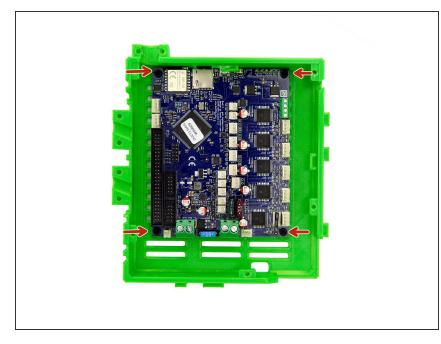
Finally, the Duet Board is attached to the Duet Box using 4x M3x8mm Hexagon Socket Head Cap Screw.
