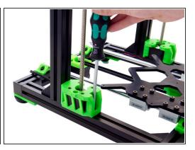
Screw the z-stepper motor to the motor mount using 4x M3x10mm Hexagon Socket Head Cap Screws.
