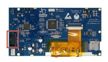
Use a 10pin ribbon cable to connect the Duet3Mini5+ to the PanelDue.
