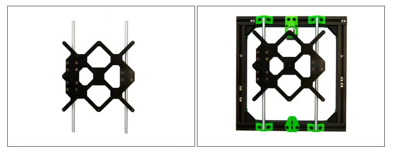
Carefully slide the 2x y-rods through the three LHBB10 ball bearings and place them on the y-rod holders.
