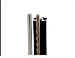
Place a z-rod in the hole next to the z-stepper motor on the z-motorholder. Carefully tap the z-rod straight into place.
