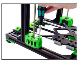
Screw the z-stepper motor to the z-motorholder using 4x M3x10mm Hexagon Socket Head Cap Screws.
