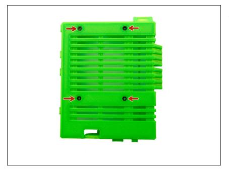
Insert 4x M3 Hexagonal Nuts (e.g. using a screwdriver or an engineer scriber) into the back of the Einsy Box.
