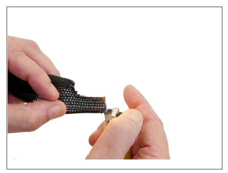
• The two ends of the Techflex tube are then briefly heated with a lighter.
