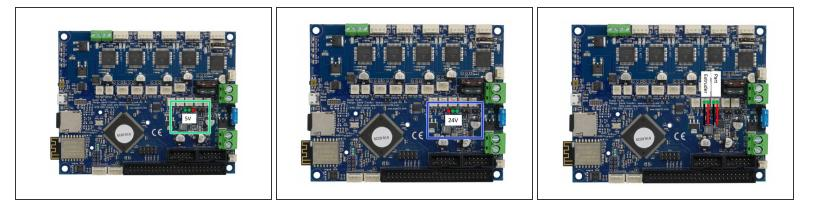
Make sure that the jumper is set according to the voltage of your fans!!!
